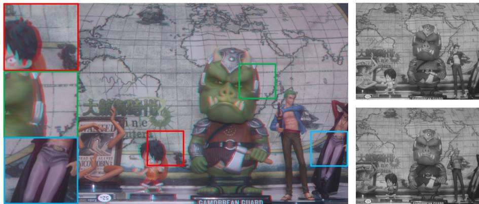
Figure 3. Left: Acquired image using the DCA camera; upper right: the red channel image; and lower right: the green channel image.
