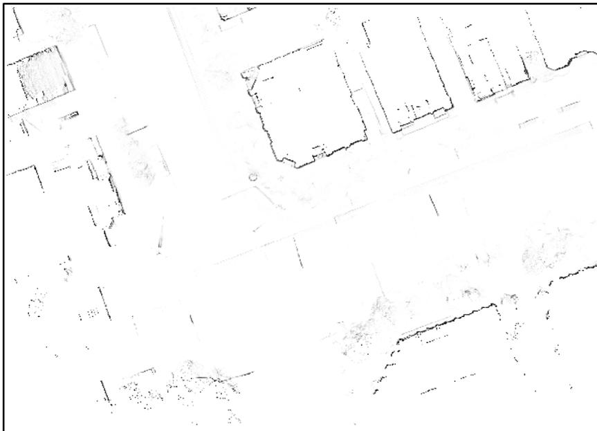
**Figure 15.** Probabilistic occupancy grid map generated by applying the IEPF algorithm.
