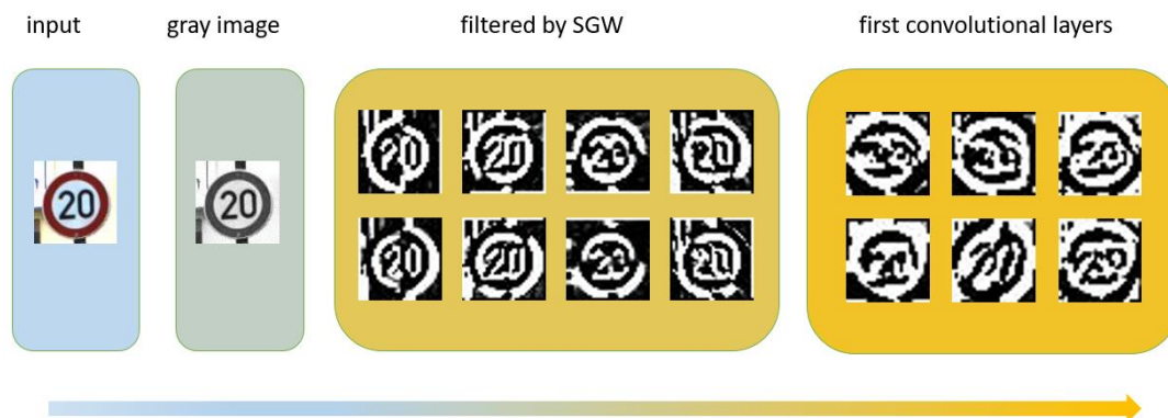
Figure 13. Visualization of the traffic sign transformation and the first convolution layers of the CNN.
