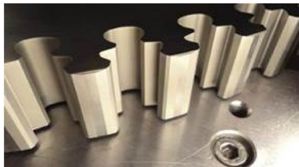
Figure 1. Example of geometry of a fir-tree slot.
