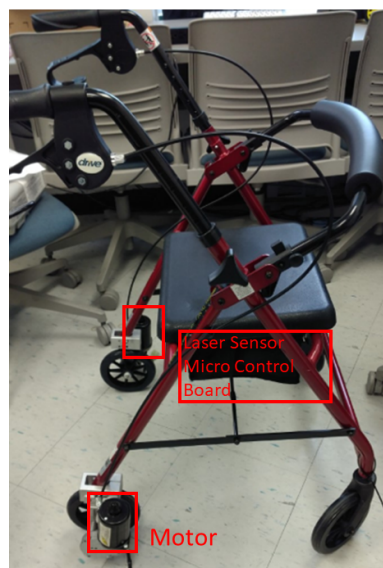
Figure 2. The motorized walker with speed control, preset course navigation, and obstacle avoidance.
