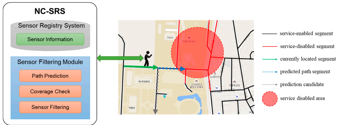
Figure 2. Concept of the network coverage information-based sensor registry system (NC-SRS) using a segment.
