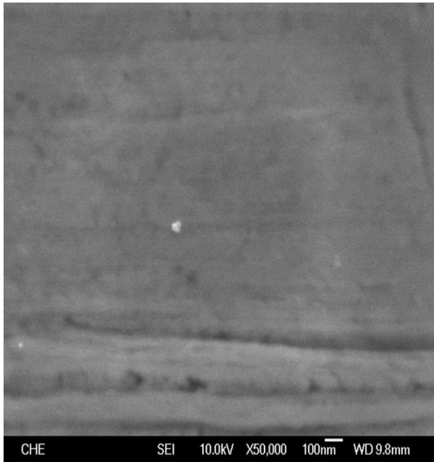
Figure S3. SEM image of PEDOT:PSS single-layer film on the Pt electrode after Au NPs immobilization.
