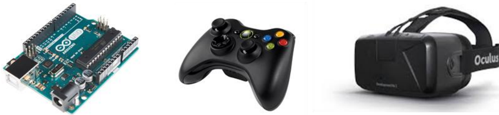
Figure 7. Hardware (input devices and output device): Arduino UNO R3, Microsoft Xbox 360, and Oculus VR DK2 from left to right.
