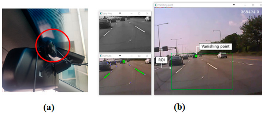
Figure 11. (a) Vision sensor; Logitech C170; (b) detected lanes and vanishing point.
