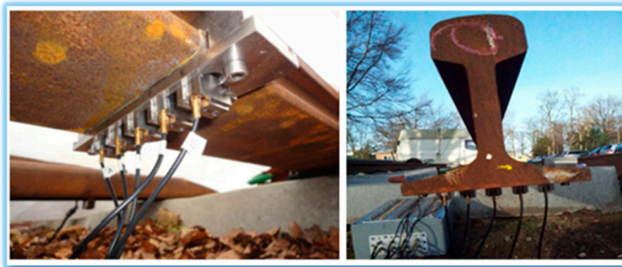
Figure 11. GWUT transducer mounting for rail foot inspections (adapted from [52]).
