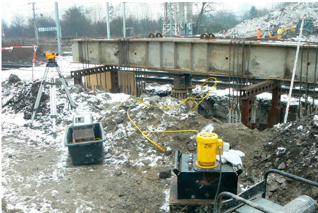
Figure 1. The basic idea of the SLT appliance with anchoring piles.
