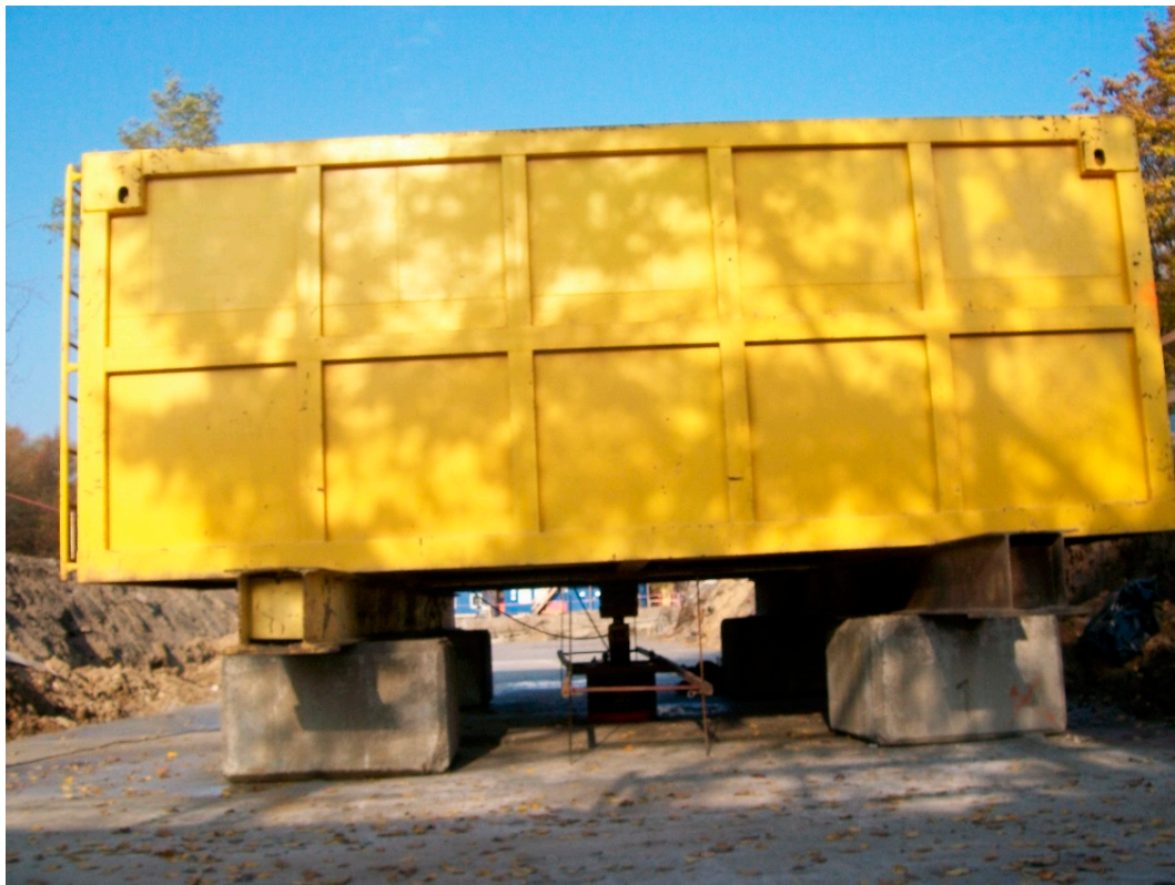
Figure 2. The SLT appliance with kentledge formed by water tanks.
