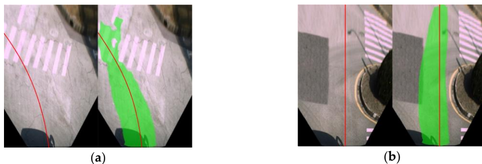
Figure 11. (a) Detection results in the presence of large cracks; (b) Detection results in the presence of inconsistent pavement colors.
