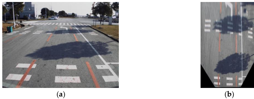
Figure 3. Images in front view and bird's-eye view: (a) Front-view image; (b) Bird's-eye-view image.
