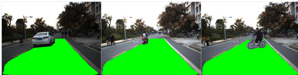
Figure 13. Detection results in the presence of various types of other road users.
