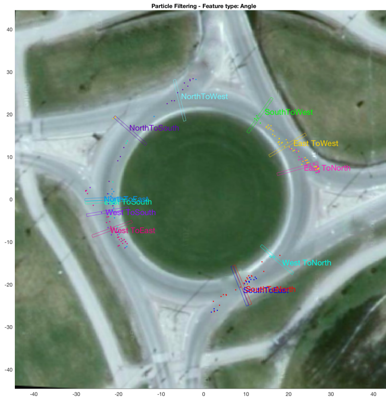
Figure 9. Aggregate results for roundabout dataset using particle filtering. The figure shows (colour-coded for each of the 12 test categories) the locations of the points beyond which 100% correct intention estimation was achieved for each test trajectory (plotted as coloured dots). The figure also shows (for each of the 12 test categories) the location of grid cell closest to the mean location of the points belonging to that category beyond which 100% correct intention estimation was achieved.
