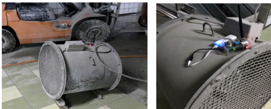
Figure 19. The interference test of sensor node.
