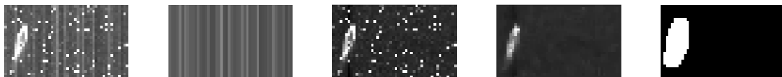
Figure 3. An example of the result of the compensation of readout dark current and detection of a stellar profile. From the left: original image, column medians, image after column compensation, outcome of median filtering, detected stellar profile.
