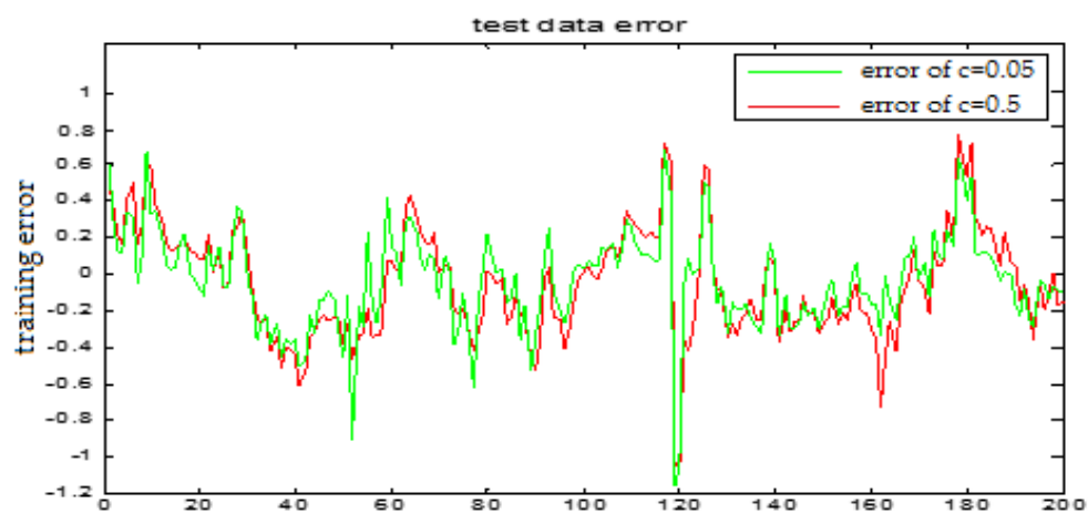
Figure 13. The TS-FNN training error curve of the central parameter c = 0.5 and c = 0.05 respectively.
