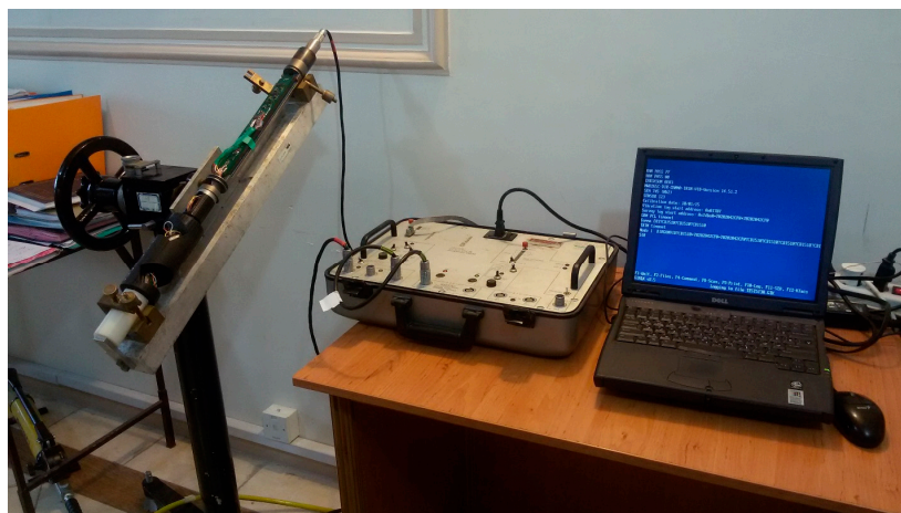
Figure 3. The tool kit with 4 redundant accelerometers, clamp, drill simulator, and monitoring system.
