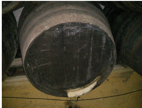
Figure 3. Wine loss due to a crack in a cask.
