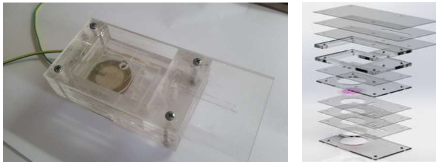
Figure 7. Top and exploded views fabricated micropump.
