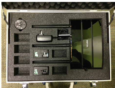
Figure 1. Building-in-Briefcase (BiB) sensor, router, and briefcase. Each briefcase can hold eight BiB sensors. By plugging in the power supply of the router, the sensors start collecting data that are forwarded to the internet data center.
