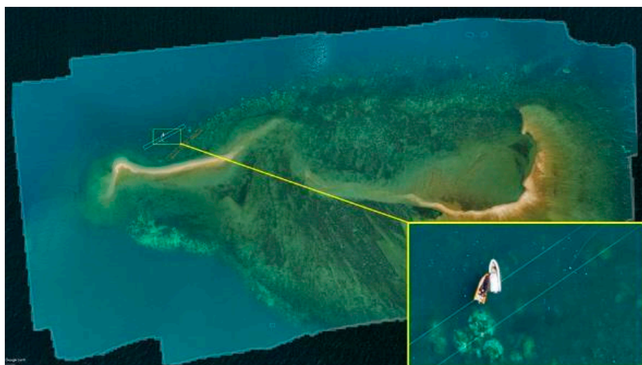
Figure 14. Photogrammetry orthomosaic of Pandora Reef (63 Ha) shows areas of day long in-water surveys performed by AIMS at the depth of 3 m (orange area) and 6 m (white area) 400% zoomed fragment on the bottom right (tide height 2.6 m).
