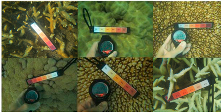
Figure 2. Example of in-water reference data with relevant bleaching level: 1 (severely bleached) to 6 (unbleached). Bleaching levels and genus from top left to bottom right: 5 Acropora , 4 Porites massive, 3 Acropora , 3 Goniopora , 2 Acropora , 1 Acropora . Courtesy of Sam Noonan (Australian Institute of Marine Science (AIMS)).
