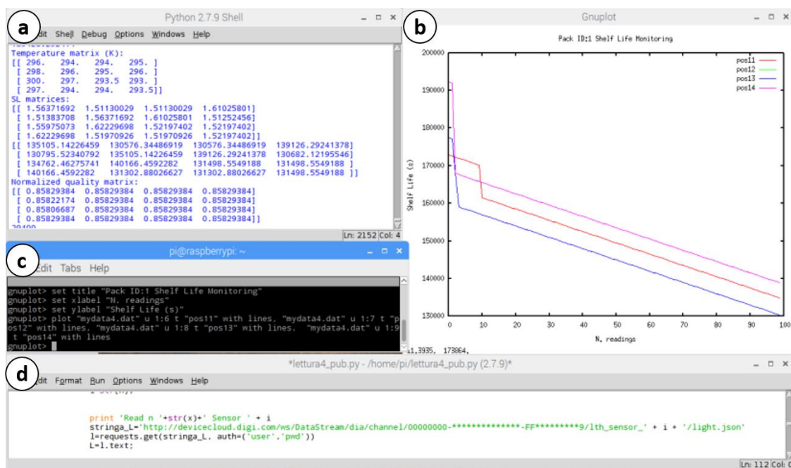
Figure 10. Screenshot of RPi-based Central Control Unit display: (a) Numeric monitoring of SL, C, T, etc. (b) Chart of SL monitoring of the selected positions for a specific pallet; (c) Chart settings panel; (d) HTTP-request panel for cloud reading.
