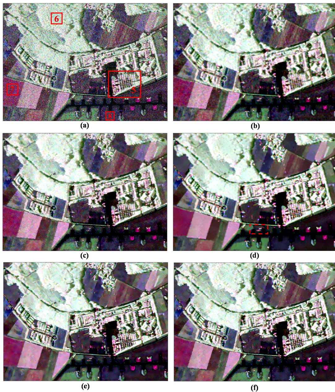
Figure 10. Denoising results of different filtering methods using ESAR L-band data. (a) Original data. (b) Refined Lee filter. (c) IDAN filter. (d) Pretest filter. (e) NL-SAR filter. (f) The proposed ANLM filter.
