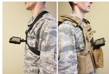
Figure 2. Smartphone Chest Mounts: velocity clip (left), juggernaut case (right).
