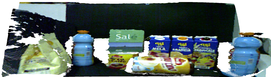
Figure 7. Representation of the dataset illustrating the scene with objects. The original point cloud used by [51] and Tombari [52] is shown in parallel projection view.
