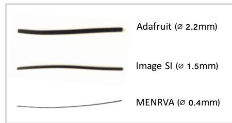
Figure 1. Comparison between the Adafruit, Image SI and Menrva sensors.
