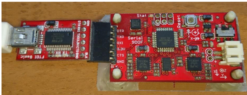
Figure 5. Low-cost microelectromechanical systems (MEMS) strap-down sensor system, SparkFun Razor 9DOF, with a serial-to-USB adapter mounted on an improvised basis.
