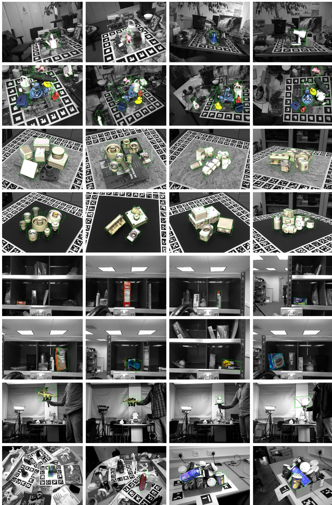
Figure 12. Proposed method results in scenes from the BOP benchmark datasets. Scene RGB data is shown in gray. Object models are shown in color and inside a green bounding box. Notice that, for scenes with multiple instances, only the most supported instance is used.
