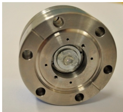
Figure 2. Bonded sapphire sample loaded in test chamber. Broadband light is focused on the center of the bonded sapphire wafer.
