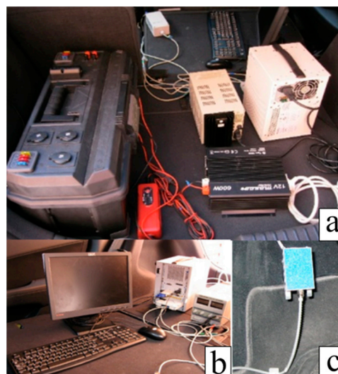
Figure 1. Power supply and devices used to convert the DC supply from the external battery to AC (a) to feed the acquisition system (b) and the force pedal (c).
