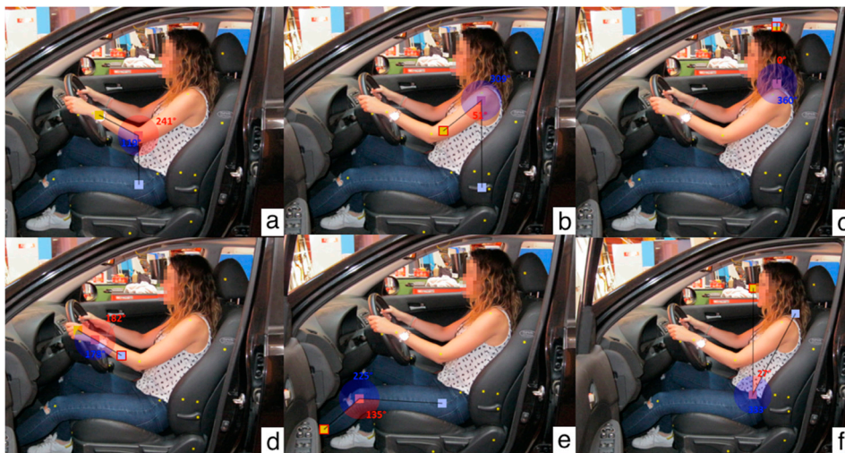
Figure 7. Examples of the limb angles of one volunteer. (a): Ankle, (b): Shoulder, (c): Neck, (d): Wrist, (e): Knee, (f): Trunk.
