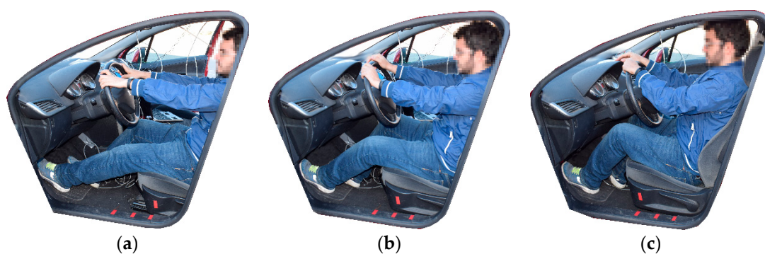
Figure 3. Position of the driver depending on the HC distance. (a) HC = 1 m, (b) HC = optimal distance, (c) HC = 0.75 m.
