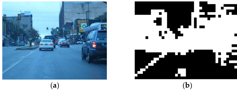
Figure 6. Sample of foreground detection result: (a) Sample frame; (b) Foreground detection result of sample frame.
