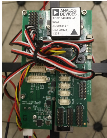
Figure 2. The ADIS16405 IMU module on the Qball-X4 quadrotor UAV.
