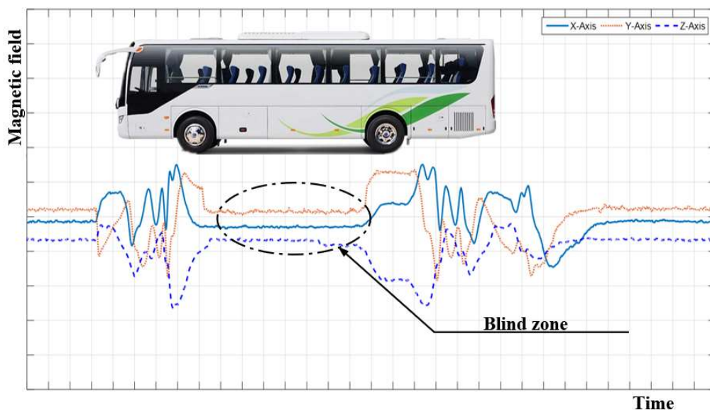
Figure 2. The magnetic signal blind zone problem of high chassis vehicles.
