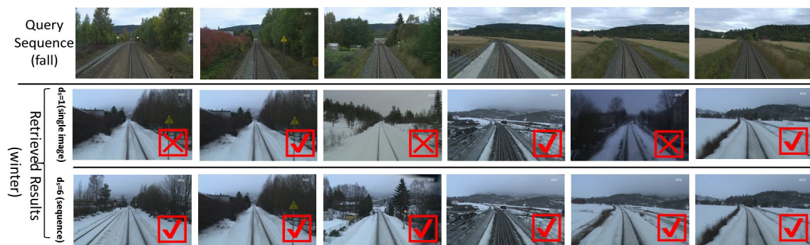
Figure 10. Frame match examples from the Nordland (fall vs. winter) data sets. The top row shows a query sequence, and the middle and third rows show the frames recalled by d_s = 1 (single image) and d_s = 6 , respectively. Visual recognition based on sequence matching achieves a better performance than that of a single image.
