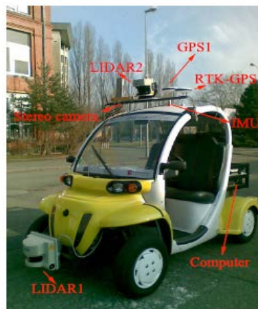
Figure 4. The experimental vehicle equipped with sensors (camera and RTK-GPS).
