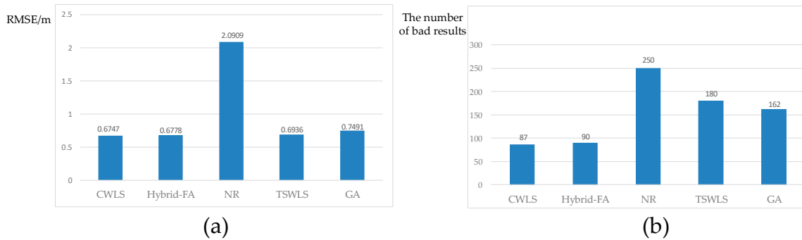
Figure 7. The results of the first experiment. (a) The RMSE of the five methods. (b) The number of bad results from the five methods.
