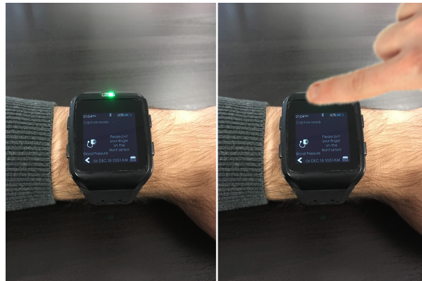
Figure 2. The CareUp ® smartwatch, where the algorithm for detecting the blood pressure (BP) has been embedded. One PPG waveform is taken from the back sensor of the watch in contact with the wrist skin and the second one is acquired by positioning the index finger of the other hand on the front oximeter sensor.
