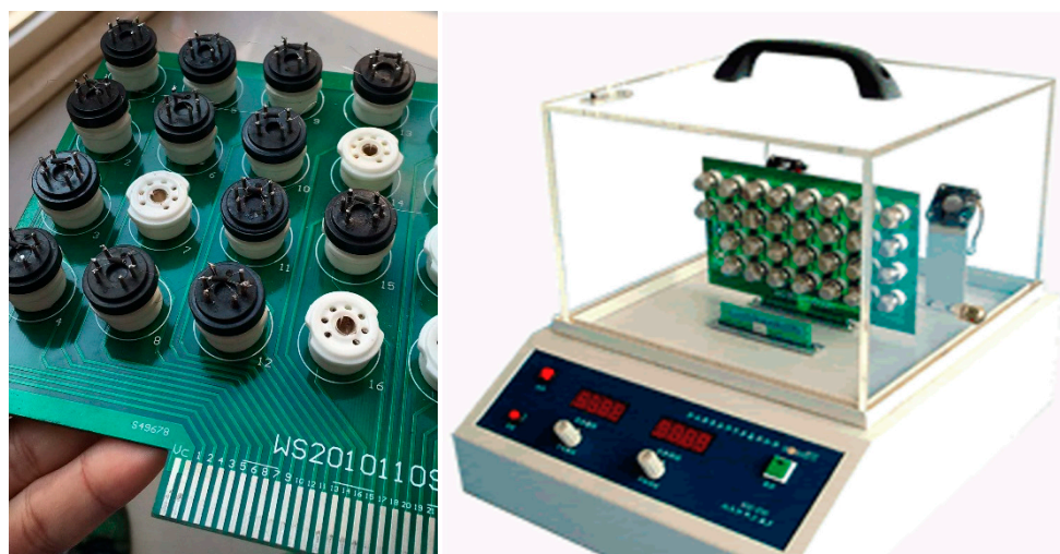
Figure S1. Photo of (a) the test circuit board and (b) the HW-30A gas-sensing test system.
