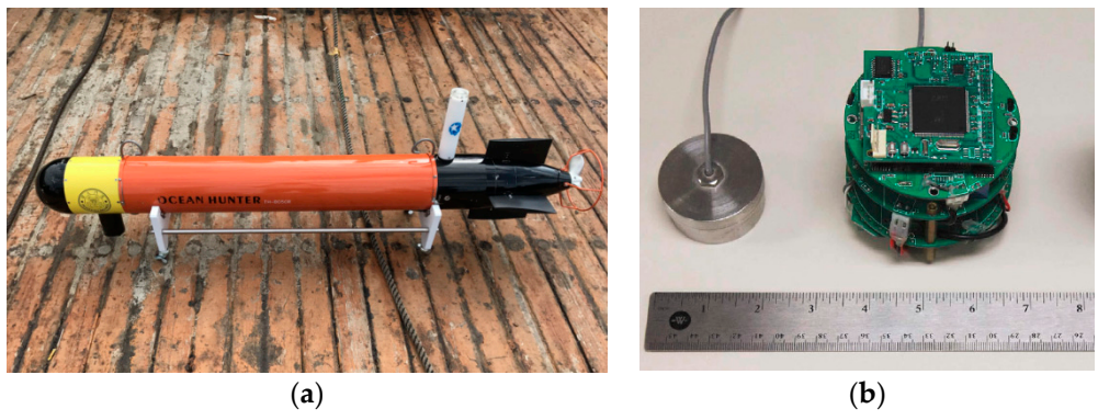
Figure 10. The autonomous underwater vehicle (AUV) and the acoustic modem module (a) The TH-050B AUV (b) The acoustic modem module.
