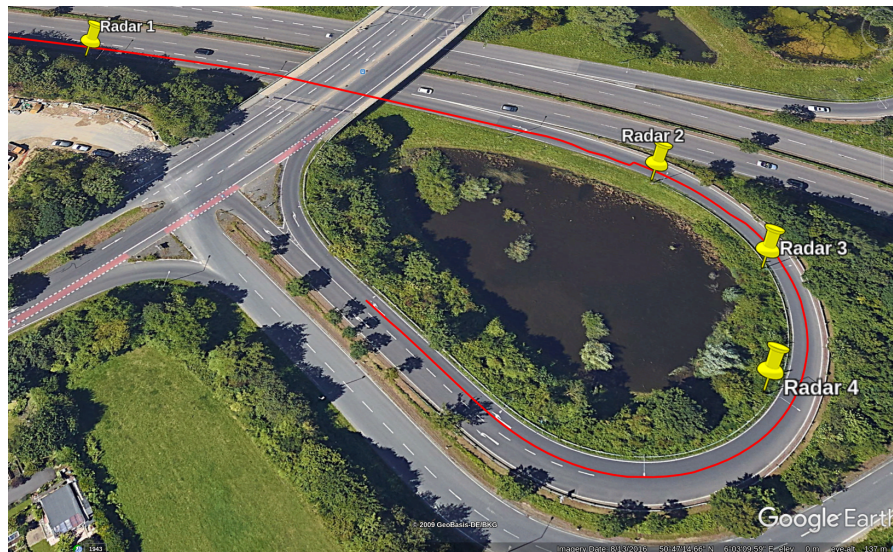
Figure 4. The location of the data recording. Four radar devices were installed at the poles marked here with yellow. The red line shows a path recorded with an RTK-GNSS sensor mounted on a vehicle.
