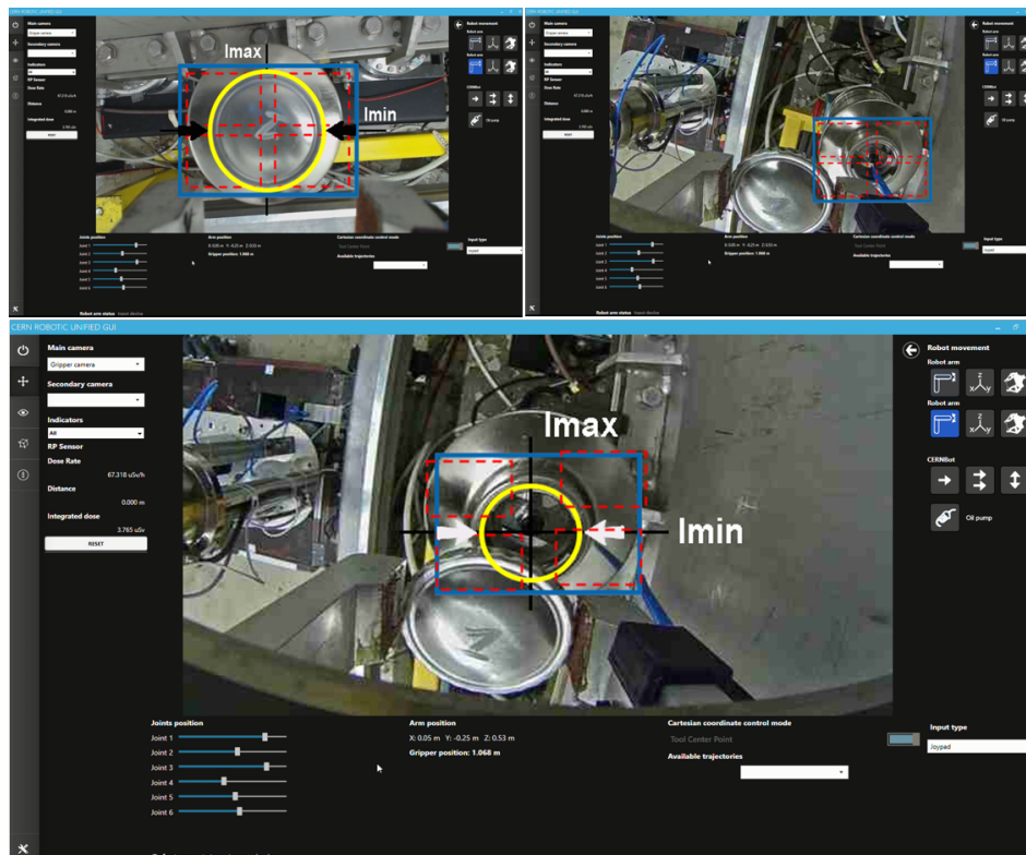
Figure 22. Grasping Determination calculation on a rounded and symmetric metallic object (radial symmetry).
