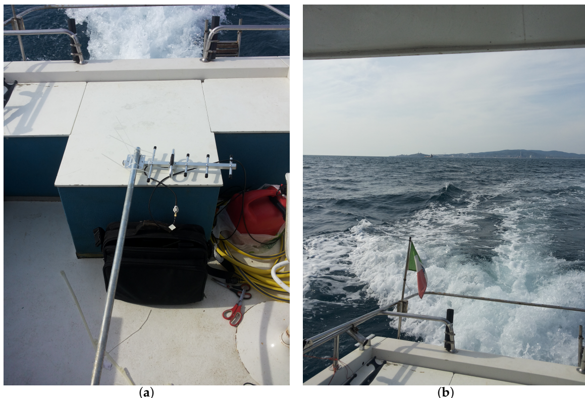
Figure 5. Offshore setup for the measurements campaign: (a) offshore end node antenna and its pole; (b) view approaching the tests spot.
