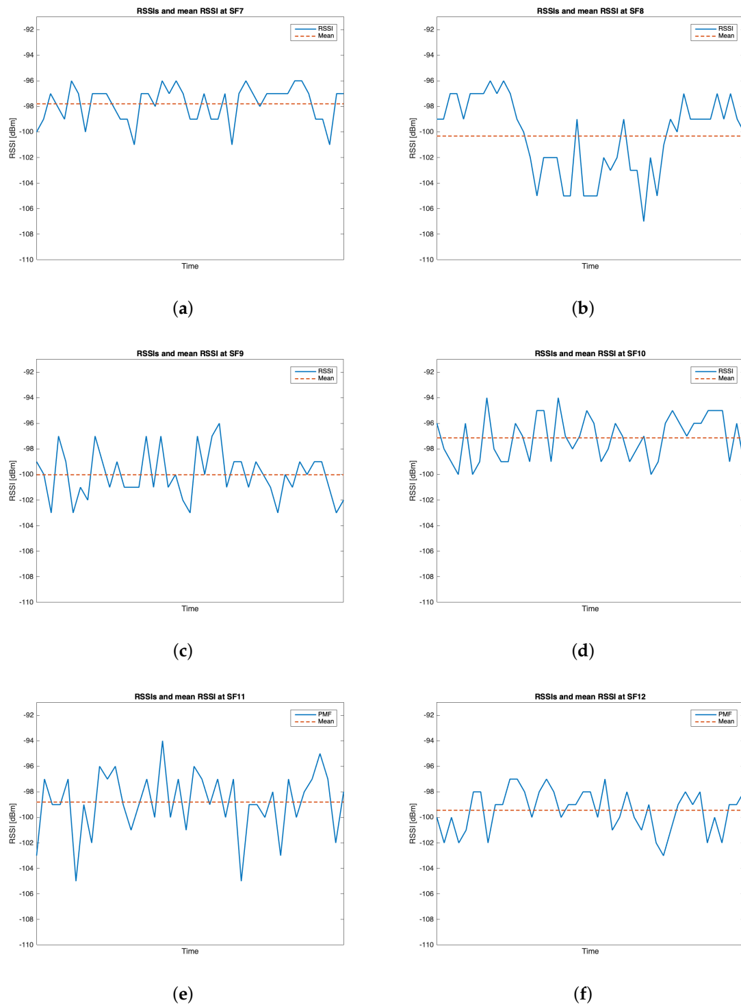
Figure 11. Group #1 RSSIs temporal trend: (a) SF = 7 ; (b) SF = 8 ; (c) SF = 9 ; (d) SF = 10 ; (e) SF = 11 ; (f) SF = 12 .
