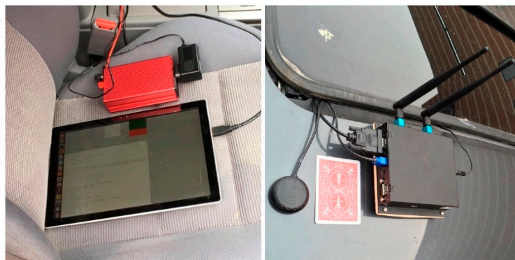
Figure 2. DSRC on-board unit (OBU), GPS antenna, and additional micro-controller (Raspberry Pi) in the DSRC network vehicle experiments.
