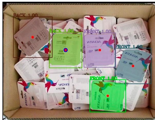
**Figure 25.** Result after calculating the center points (red points) and deciding the final target (blue point).
