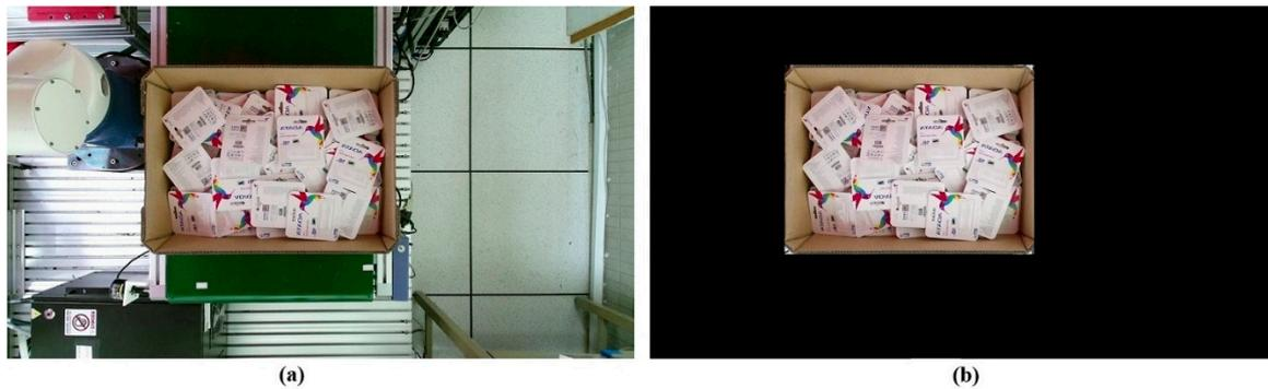
**Figure 22.** Image preprocessing to remove unnecessary information—(a) the original RGB image captured by the camera; (b) the result after removing the unnecessary information.
