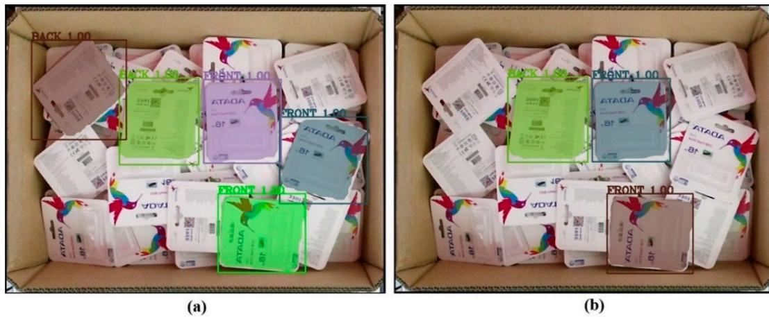
**Figure 24.** Result after passing through the filter at a fixed area threshold percentage criteria: (a) 90%, (b) 95%.
