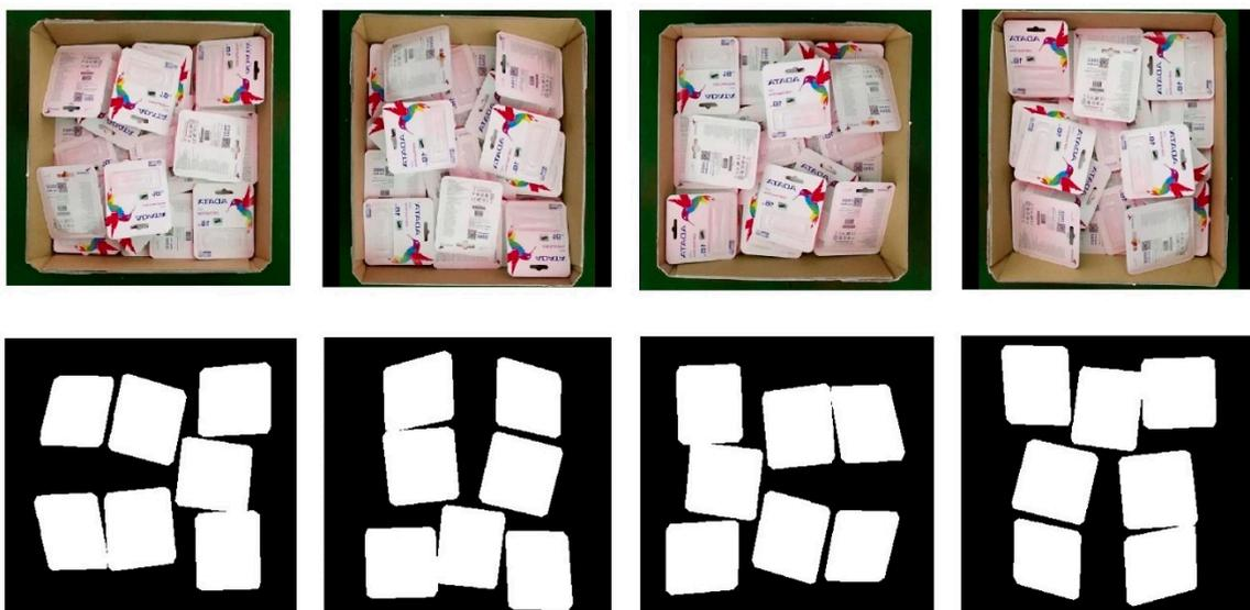
Figure 4. **Top:** Original image and three other versions after the original data passed through the augmentation module. **Bottom:** Corresponding binary image.
