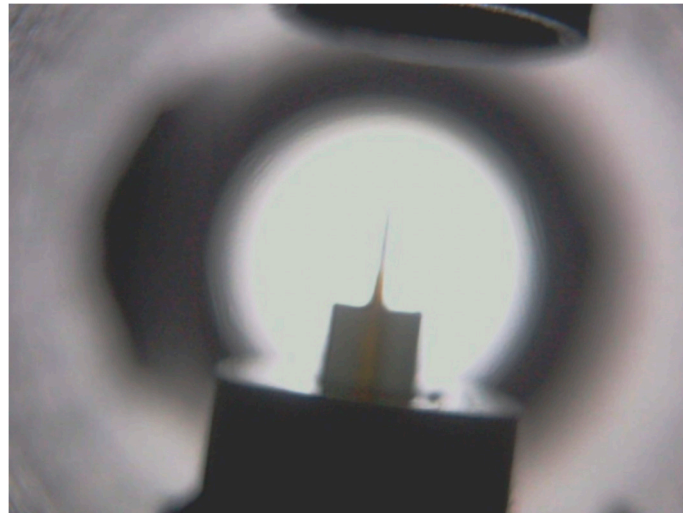
Figure 2. Inside of the electrospray chamber. The tip of the quartz-capillary is seen in the center.
