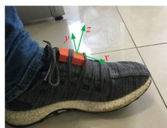
**Figure 3.** The inertial navigation system (INS)-based foot-mounted PDR system.
