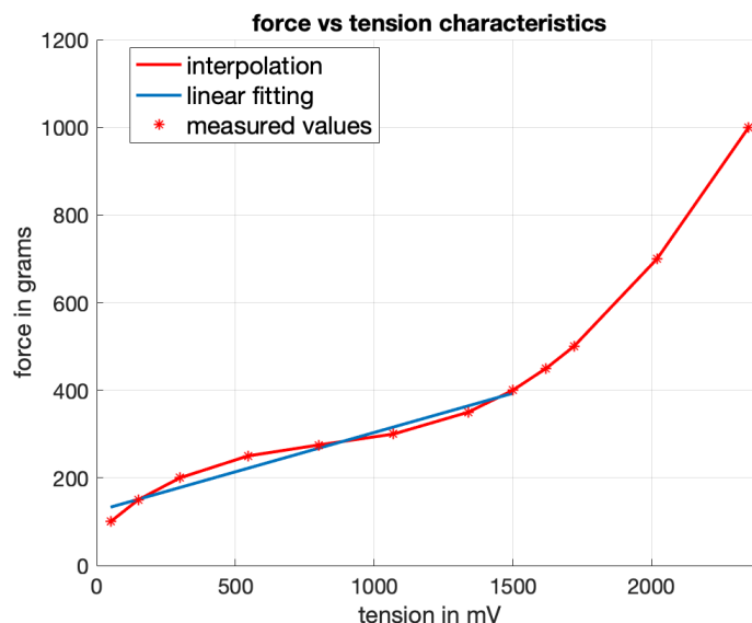
Figure 5. Static force in grams as a function of the tension output in mV of the sensors. The relation is almost linear between 50 and 1500 mV.
