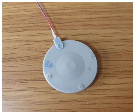
Figure 12. Photograph of the prototype cymbal transducer coated for measurement in water.
