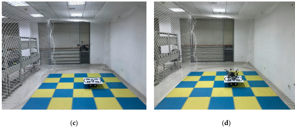
Figure 11. Autonomously approaching (a,b), descending (c), and landing on a static landing pad (d).
