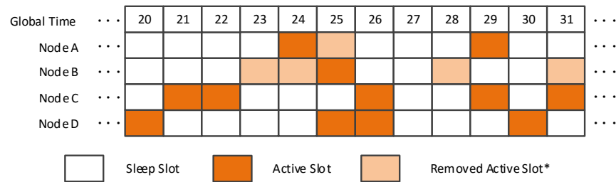
Figure 2. VN-NDP when the pairwise method is Disco. VN-NDP: A neighbor discovery protocol based on virtual nodes. (*A removed active slot means a sleep slot that is an active slot in the original wake-up schedule).
