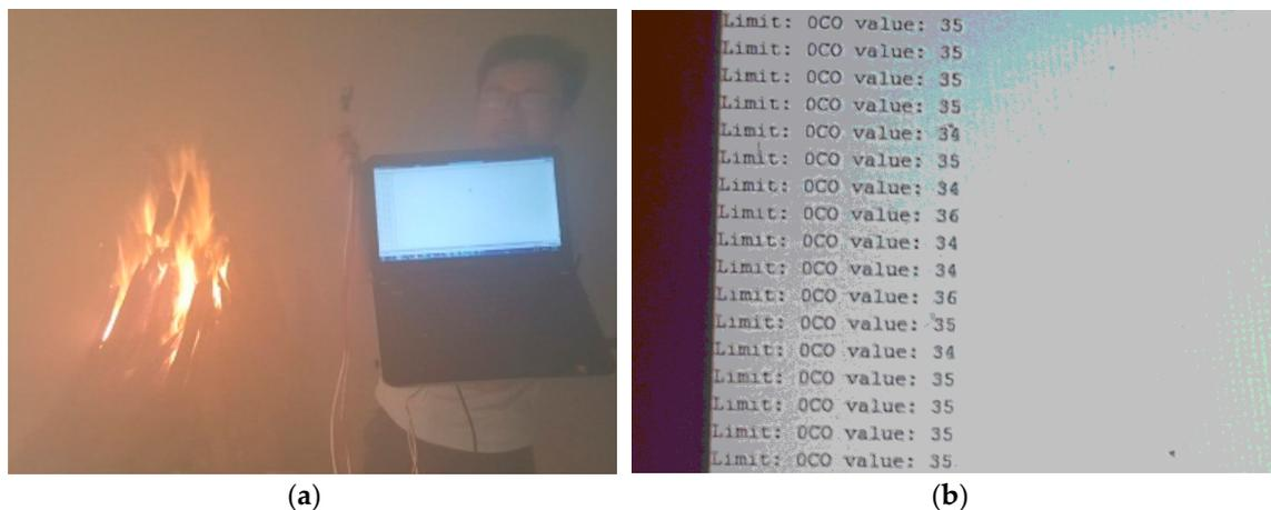
**Figure 14.** (a) Testing and measuring the CO level in the fire; (b) the measured CO values.
